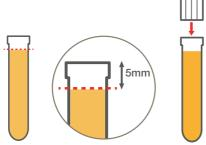
It is good practise to shake the sample before measurement as samples can settle with time – if the ferrous material is not evenly mixed throughout the sample, the FWM+ may over, or under report the ferrous content of the sample.
